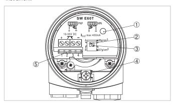
Electronics and terminal compartment, single chamber housing
