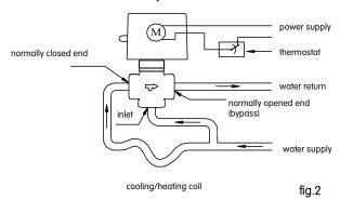
3-way diverting valves: inlet is the normaly closed end and the normally open end is the bypass port (the inlet
