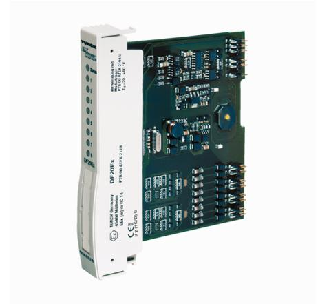
The input module DF20EX is equipped with 8 channels according to NAMUR which are split into two blocks. There is one frequency input per block and three control inputs/outputs.
