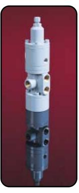
Designed for pneumatic systems, Conoflow Series GVB Snap-Acting Relays change ports to switch or lock in secondary air source when the main supply pressure fails below a predetermined set point. In the event of supply or pilot pressure failure, the positive action relay with one common and two inlet or outlet ports will automatically:
