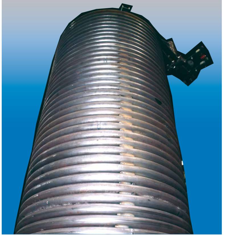
GMT EG is a multi-function steam or hot water exhaust gas economizer is a water tube, forced circulation boiler for heat recovery of diesel and gas engine exhaust gas. The heat transfer surface consists of concentric, parallel steel tube coils connected to inlet and outlet manifold pipes.
