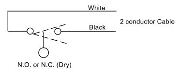
**To Select Switch Operation** ... LS-270 units are supplied with SPST switch N.C. or N.O. (dry). To convert switch operation: Remove grip ring and cap from unit, invert float on stem and reassemble unit.
