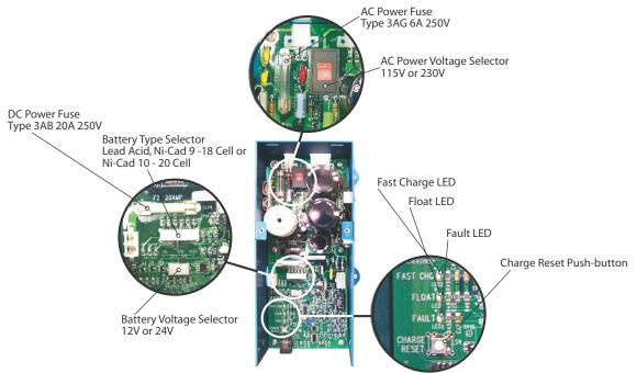
The Firetrol® battery charger features a fully automatic 4 step charging cycle. The charging cycles are as indicated:
