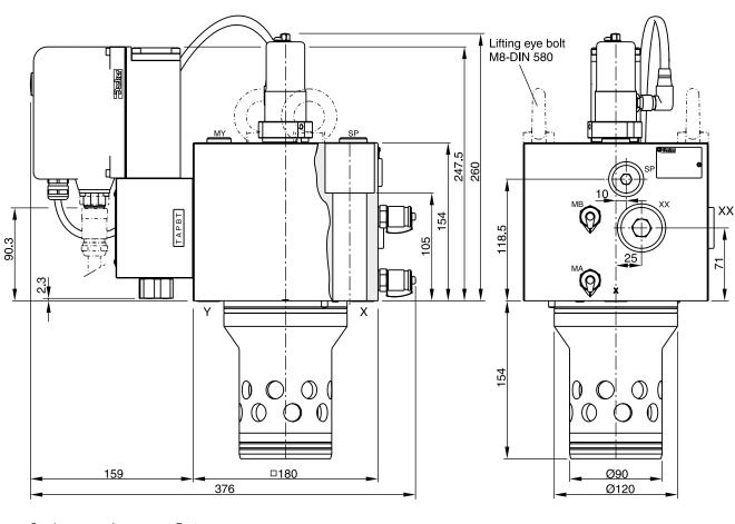
$\begin{array}{ll} \text{Suction port} & \text{Accu port} & \text{Ports} \\ \text{SP} = G1/2" & \text{XX} = G3/4" & \text{MA and } \text{MB} = G1/4" \\ \end{array}$
