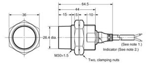
Note 1. 4-dia. vinyl-insulated round cable with 3 conductors (conductor cross section: 0.3 mm<sup>2</sup>; insulator diameter: 1.3 mm); standard length: 2 m 2. Operation indicator (yellow)
