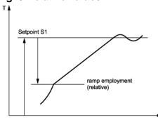
The main setpoint S1 and the point of ramp employment are linked as difference with one another. This difference can take positive or negative values, i.e. starting point for the ramp can be above the setpoint at cooling function or below the setpoint at heating function, and automatically runs along with adjustments of the desired value.
