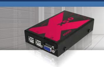
High density, small form factor, VGA extension over CATx cable
