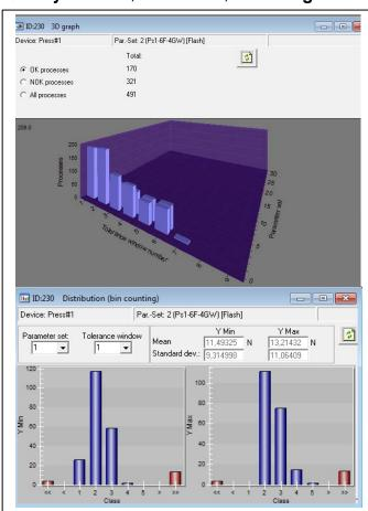
Quality and tool wear for the fitting process can be assessed using the statistics functions.
