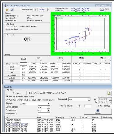
With the MP85A(DP), it is possible to store results, curves, statistics and the device settings. This allows processes to be analyzed later on and ensures 100% traceability.
