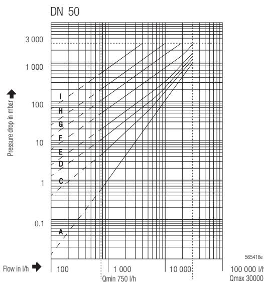
Recommended pressure drop max. 1 bar
