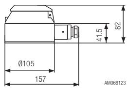
High resolution INA inductive pulser according to IEC 60947-5-6,
