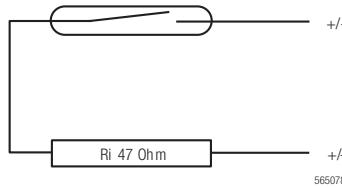
This simple version of a reed pulser is suitable for remote totalizing. For industrial control systems the IN or INA versions are recommended. Electronic pulse counters have low switching power consumption. They are therefore energized directly from the pulser. Electromechanical pulse counters with power consumption exceeding 2 W require an intermediate switching relay (e.g. WE 77).
