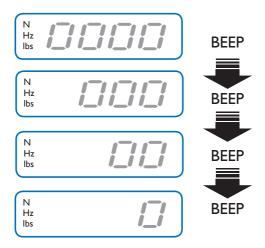
If these signals are seen and heard, batteries should be replaced. Batteries are accessed through the removable cover on the back of the meter. New batteries should be inserted within 30 seconds of removal of old batteries. Taking longer risks loss of any data stored by the memory keys. Batteries are expected to provide approximately 20 hours of continuous operation before replacement is required when the optical sensor is used. Over 100 hours of use is possible when the acoustic sensor is used.
