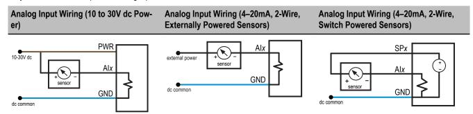
(Only possible in models with switch power (SPx) outputs)
