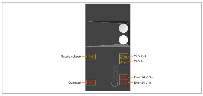
Figure 1: Auxiliary supply modules with 24 V Out and 24 V In (8B0C0320Hx00.00A-1) - Status indicator groups
