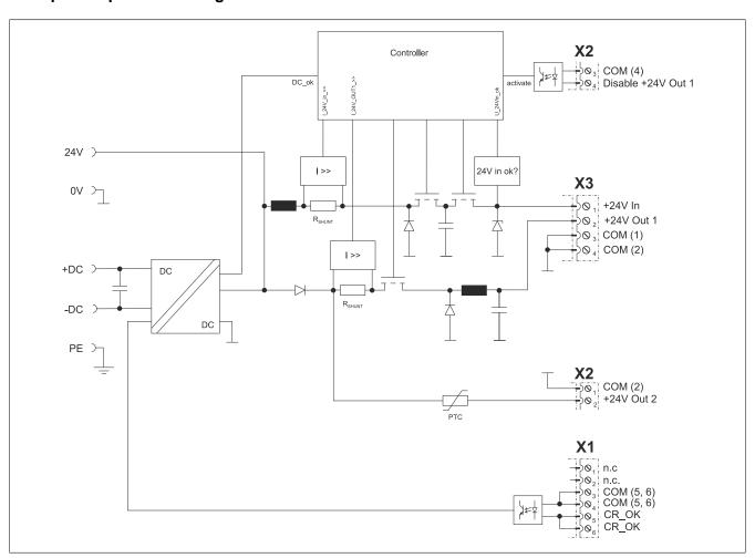
Figure 4: 8B0C0320Hx00.00A-1 - Input/Output circuit diagram
