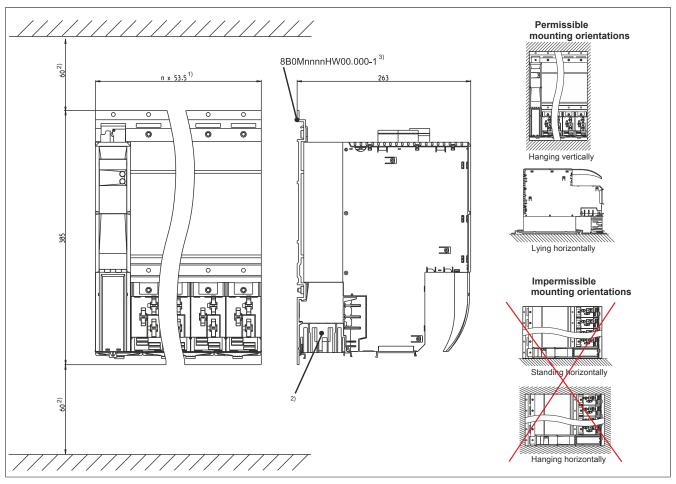
Figure 2: Dimension diagram and installation dimensions
