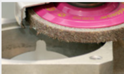
Aluminium: for cleaning and fine grinding
