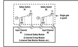
The non-safety contact (33/34) will switch at a greater degree (rotation) than the safety contacts and may not indicate if the guard is slightly open (see *Figure 3* on page 1). In such situations, an unused safety contact can more accurately indicate the status of the guard.
