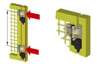
Figure 4. Hinge Switch Installation
