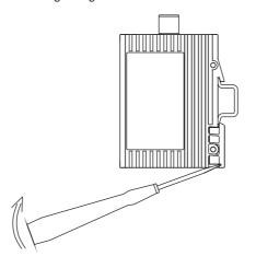
Fig. 7: Dismantling the SPIDER xTX(/xFX)
