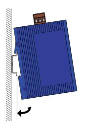
Fig. 5: Assembling the SPIDER xTX(/xFX)
