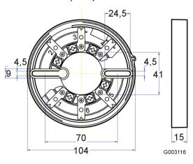
UB-6 is prepared for SUM-2 assembly. Detectors in the CN, EV and EVC series can be locked to the base using a 1,5 mm hexagon key.
