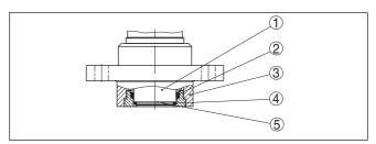
Fig. 7: Front-flush installation of the measuring cell with double seal (example: flange connection with extension)
