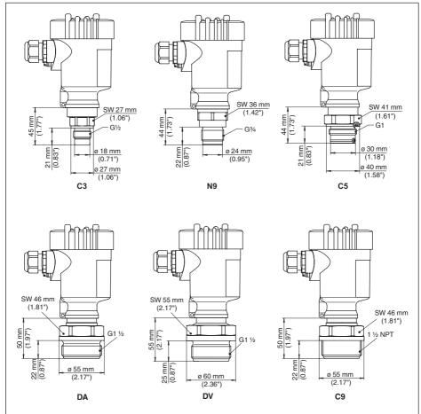
Fig. 47: VEGABAR 82, threaded fitting front-flush
