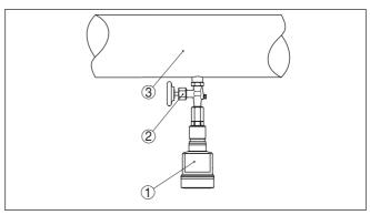
Fig. 17: Measurement setup for process pressure measurement of liquids in pipelines
