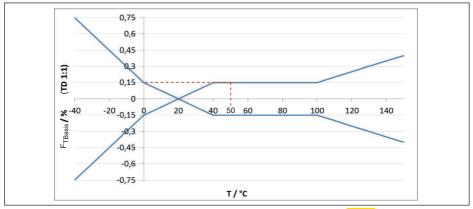
Fig. 43: Determination of the basic temperature error for the above example:  $F_{TBasis} = \frac{0.15 \%}{0.15 \%}$
