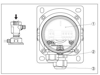
Fig. 27: Electronics and terminal compartment
