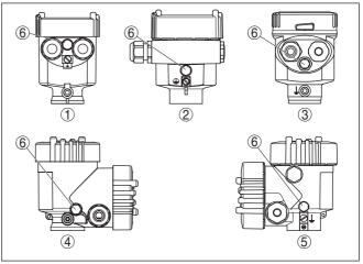
Fig. 11: Position of the filter element - non-Ex, Ex-ia and Ex-d-ia version
