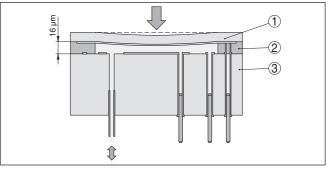
Fig. 3: Configuration of the CERTEC® measuring cell
