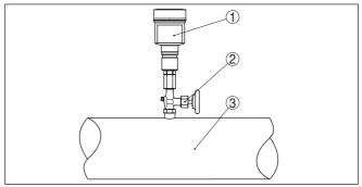
Fig. 15: Measurement setup for process pressure measurement of gases in pipelines
