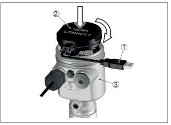
Fig. 34: Connection of the PC directly to the sensor via the interface adapter
