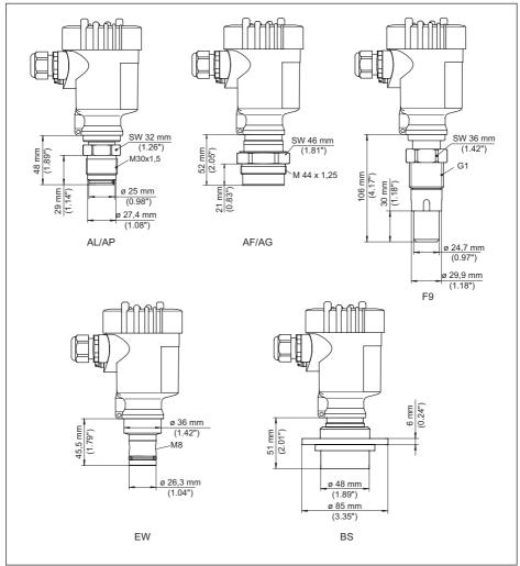
Fig. 50: VEGABAR 82, extension fitting
