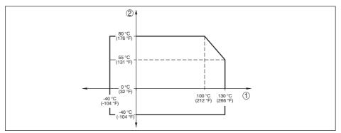
Fig. 41: Temperature derating VEGABAR 82, version up to +130 °C (+266 °F)
