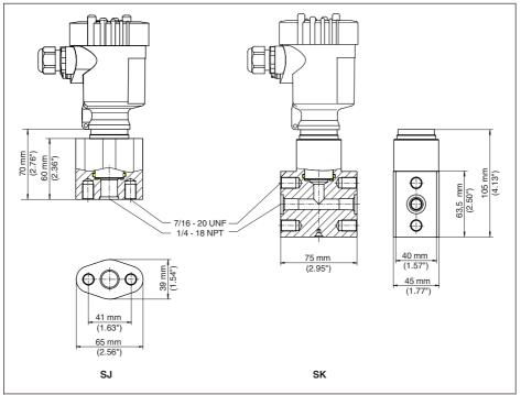
Fig. 52: VEGABAR 82, connection acc. to IEC 61518
