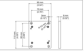
Fig. 20: Drilling template - wall mounting plate
