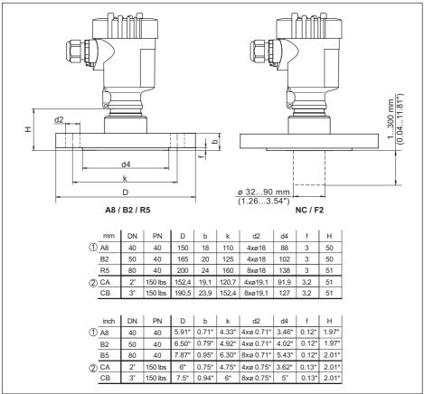
Fig. 49: VEGABAR 82, flange connection
