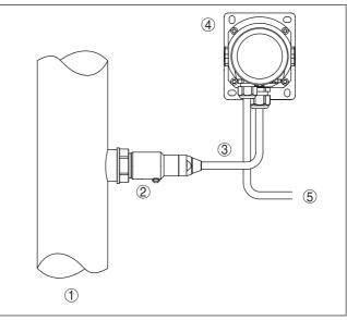
Fig. 19: Configuration, process module, external housing
