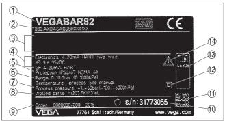
Fig. 1: Layout of the type label (example)
