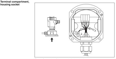
Fig. 28: Connection of the sensor in the housing base
