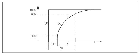
Fig. 38: Behaviour in case of sudden change of the process variable.  $t_{\tau}$  dead time;  $t_{A}$ : rise time;  $t_{S}$  jump response time
