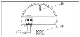
Fig. 24: Electronics and terminal compartment - single chamber housing
