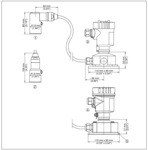
Fig. 45: VEGABAR 82, IP 68 version with external housing
