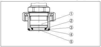
Fig. 8: Hygienic installation of the measuring cell (example: hygienic fitting with compression nut)
