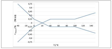
Fig. 39: Basic temperature error F<sub>TBasis</sub> at TD 1 : 1
