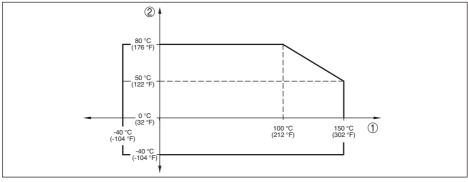
Fig. 42: Temperature derating VEGABAR 82, version up to +150 °C (+302 °F)
