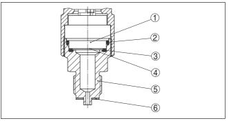
Fig. 4: Recessed installation of the measuring cell (example: manometer connection G1/2)
