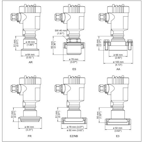
Fig. 48: VEGABAR 82, hygienic fitting
