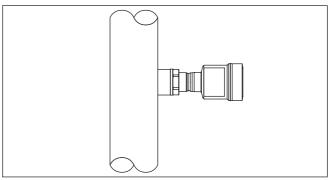
Fig. 2: Process pressure measurement VEGABAR 82
