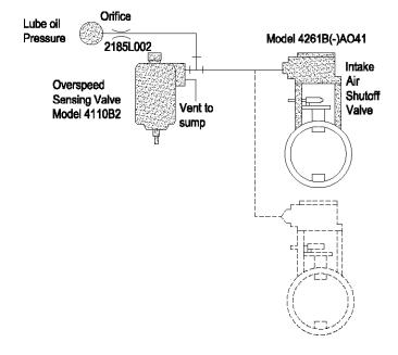
Hydro-mechanical Runaway Shutdown System
