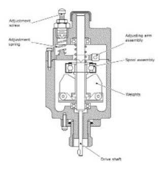
The Model 4110 Overspeed Sensing Valve uses a precision flyweight speed sensor to vent a pneumatic or hydraulic signal (via a built-in two-way valve) at a pre-set RPM.
