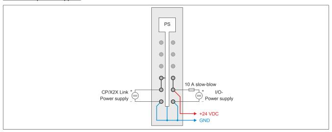
Figure 6: X20 CPUs - Connection example with two separate supplies
