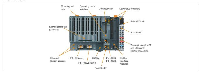
Figure 1: X20 CPUs - Operating elements for X20CP1483, X20CP1483-1, X20CP1484, X20CP1484-1, X20CP1485, X20CP1485-1 and X20CP1486
