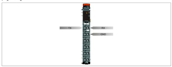
Figure 8: X20 CPUs - Pinout - RS232 interface (IF1)
