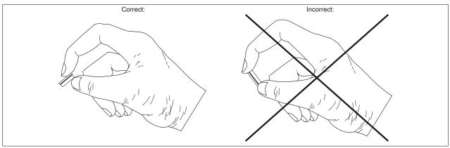
Figure 14: X20 CPUs - Correct grip for the battery
