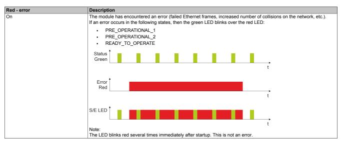
Table 10: Status / Error LED as error LED - POWERLINK V2 operating mode
