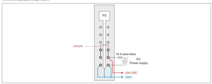
Figure 7: X20 CPUs - Connection example with a supply and jumper
