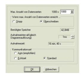
1) Polling Mode = Method, to determine the status of a device consisting of hardware or software or the event of a change of values by cyclic queries.
