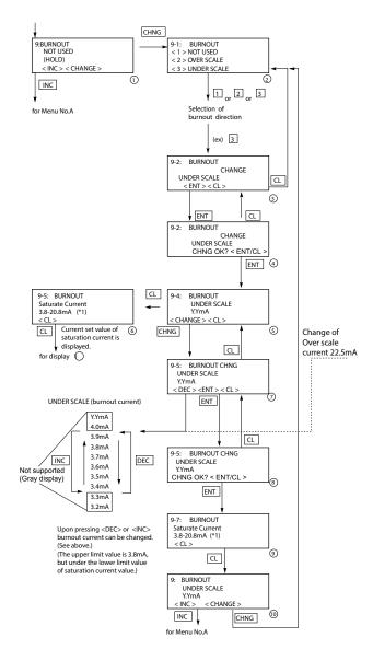
\*1) When it's NAMUR sepecification, the saturation current is 3.8~20.8mA
