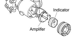
Check all the screws are correctly tightened, and screw the electronics housing cover on the transmitter
