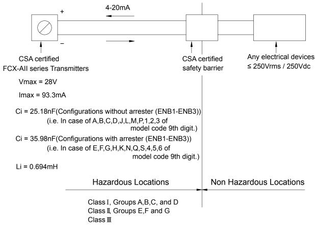
Temp. Code T4 ( $T_{amb} = 70^{\circ}C_{max}$ ), T5 ( $T_{amb} = 50^{\circ}C_{max}$ )
