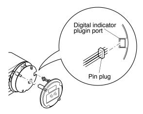
(5) Fasten the digital indicator to the electronics section by tightening 2 fixing screws.
