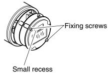
(6) Assemble the electronics housing cover.
