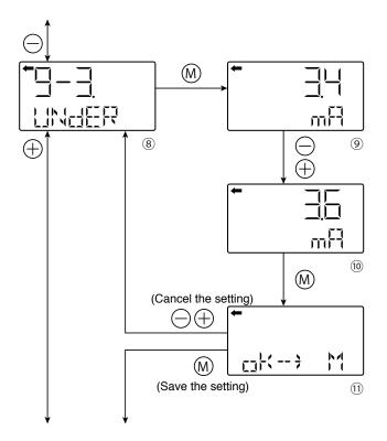
**9-3 UNDER : Change of burnout current** when UNDER (UNDERSCALE) is selected.
