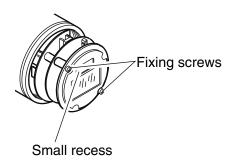
(6) Assemble the electronics housing cover.
