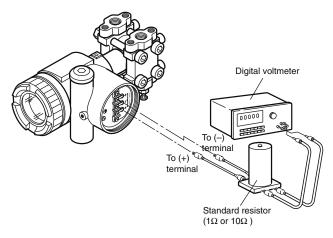
Output measurement on the current loop (4/20 mA)
