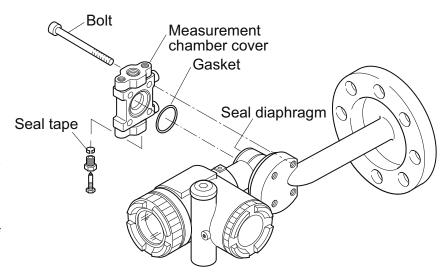
(5) Reassemble the detecting unit by reversing the disassembling procedure.
