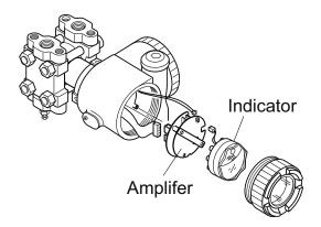
Check all the screws are correctly tightened, and screw the electronics housing cover on the transmitter
