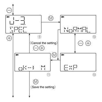
J-3 SPEC : Selection of the burnout & saturation current value specification (normal specification/expanded specification)
