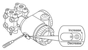
(3) Adjust zero point (4 mA) by turning the external screw
