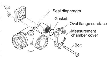
(5) Reassemble the detecting unit by reversing the disassembling procedure.
