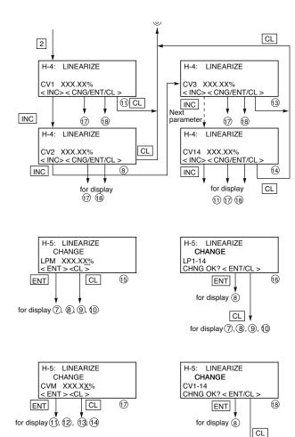
When ENT is pressed at display of ②, the following is displayed,
