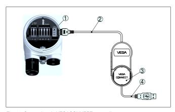
Fig. 18: Connection via VEGACONNECT externally
