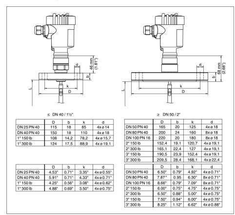
Fig. 30: VEGAFLEX 65, flange version
