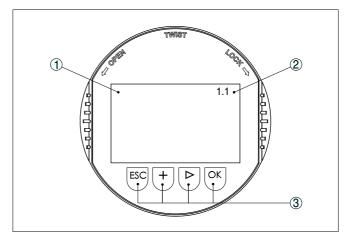
Fig. 16: Indicating and adjustment elements
