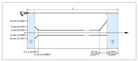
Fig. 22: Deviation VEGAFLEX 65 in coax version in oil
