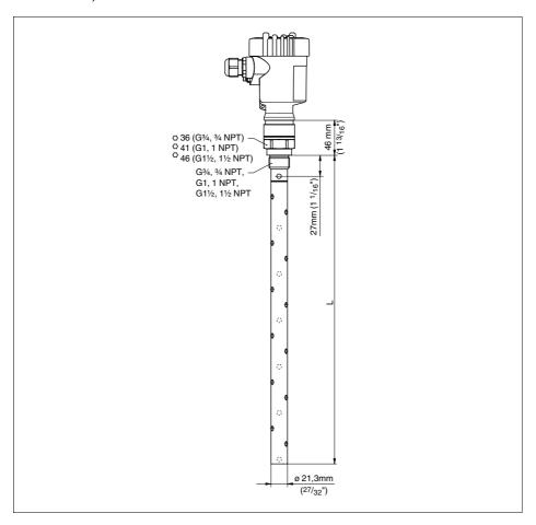
Fig. 29: VEGAFLEX 65, threaded version
