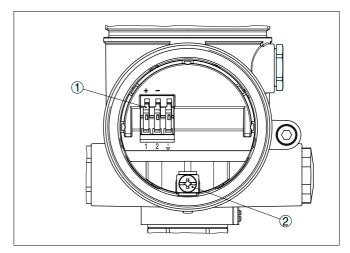
Fig. 12: Connection compartment, Ex-d double chamber housing
