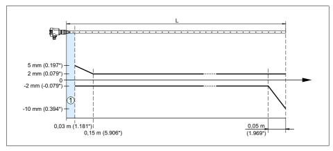
Fig. 21: Deviation VEGAFLEX 65 in coax version in water
