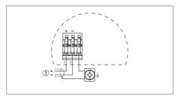
Fig. 13: Wiring plan, Ex-d double chamber housing
