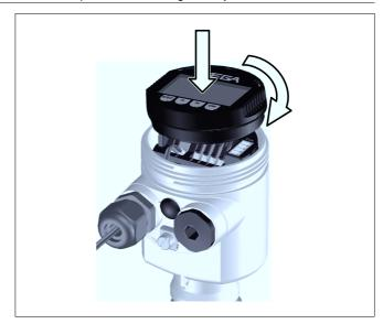
Fig. 15: Insert indicating and adjustment module
