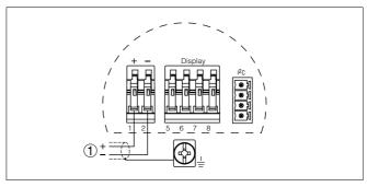
Fig. 7: Wiring plan, single chamber housing
