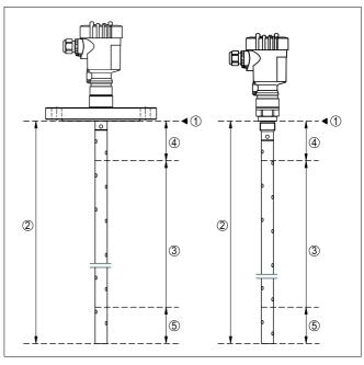
Fig. 20: Measuring ranges of VEGAFLEX 65
