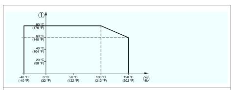
Fig. 23: Ambient temperature - Process temperature
