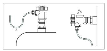
Fig. 2: Measures against moisture penetration
