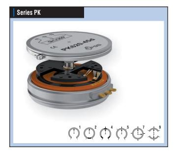
Resistance elements of **conductive plastic**, imprinted on glass-fiber reinforced supports. The max. active angle amounts to 355°. Smaller angles, tappings and shorted sections on request.
