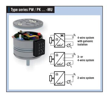
**Angular position transducers**, equipped with resistance elements of wire or plastic resistance elements with integrated R/I or R/V converter for current or voltage output, optional with a configuration of 2, 3 or 4 wires.
