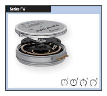
Resistance elements as **straight winding** with wire winding on a coated former of copper wire are used in potentiometers of the multiple-turn or linear type but also in single-turn potentiometers with active angles up to max. 350°.
