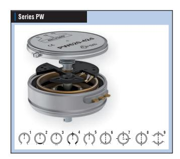
Resistance elements as **ring winding** with wire winding on an anodised aluminium anchor ring can be provided with any circuit, angle and resistance values.
