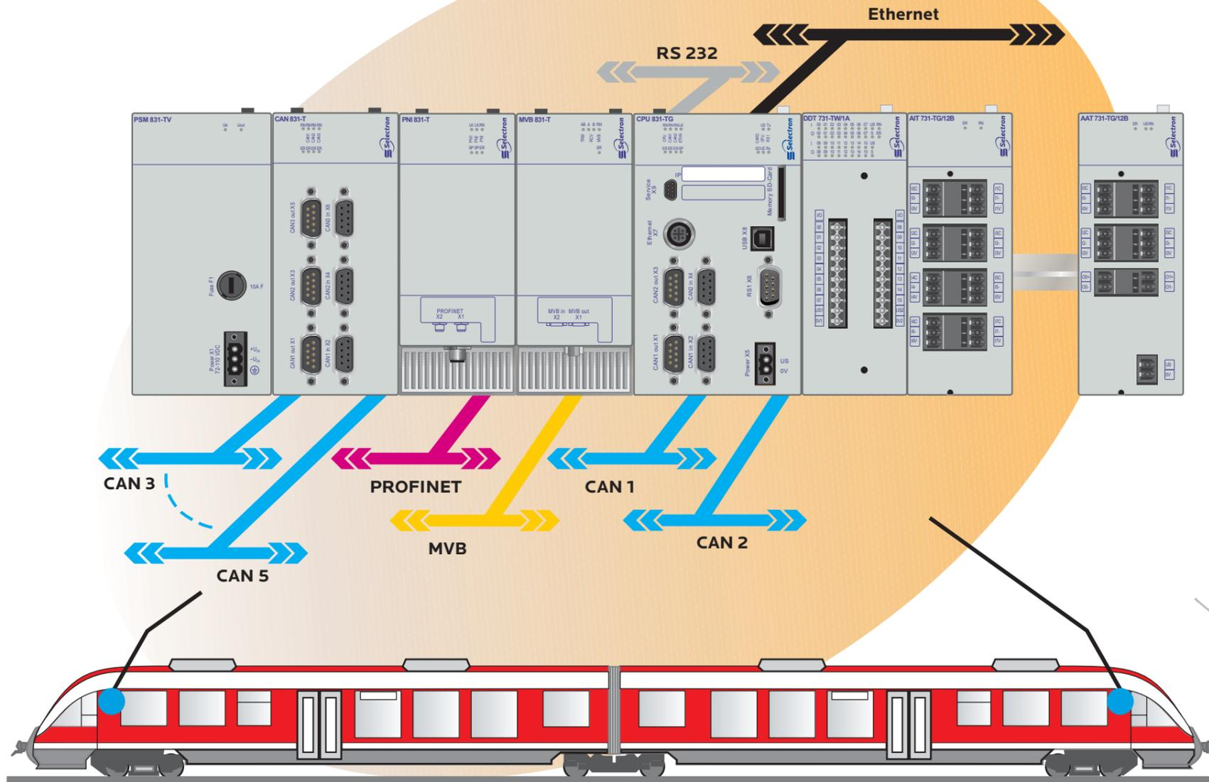
The **Selectron® MAS 83x-T** vehicle control unit can be used as a **standalone** unit with decentralized, via **CAN connected** extensions or with local **I/Os** and **communication interfaces** or mixed using both.
