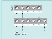
The DMxx can also be controlled using the JOVENTA Positioner (PA/PF) with control signal of DC 0...10 V.
