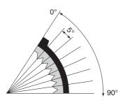
The limitation or rotation angle can be set in 5° steps by moving the adapter.
