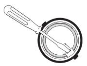
The adapter can be remove simply by pressing the adapter clip on the underside of the actuator
