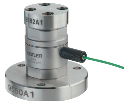
Fig. 1: Calibrating element with force distribution cap, flange and cable protector
