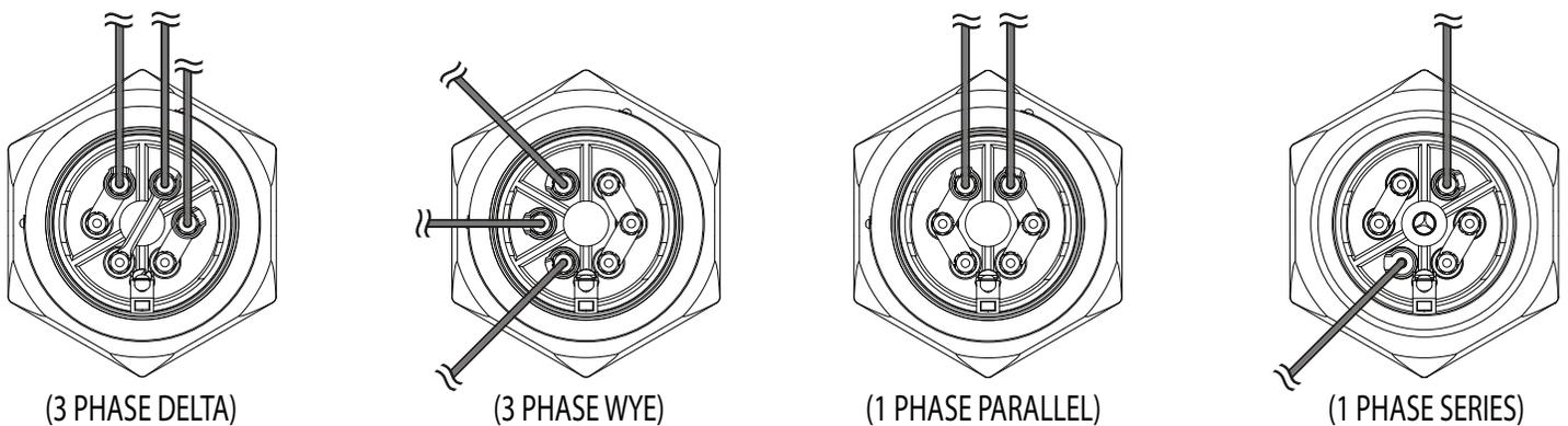
Figure 15. Heating tank element phase configurations. Replacement elements may be a different phase configuration.
