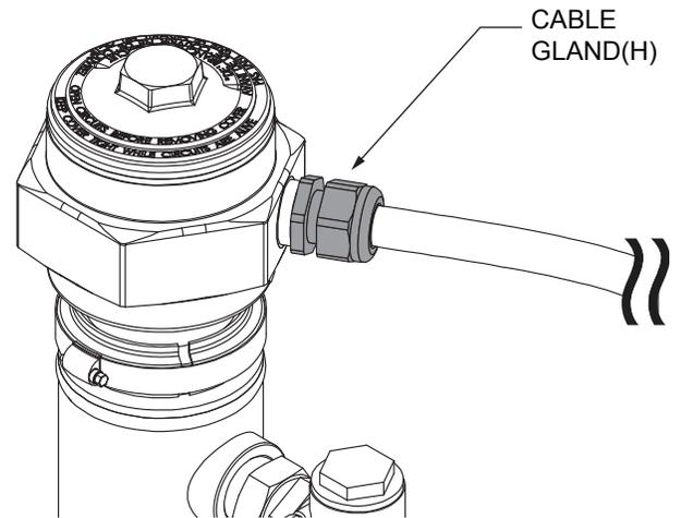
Figure 14. The cable gland as shown connected to the element assembly. Unscrew to remove element wiring.
