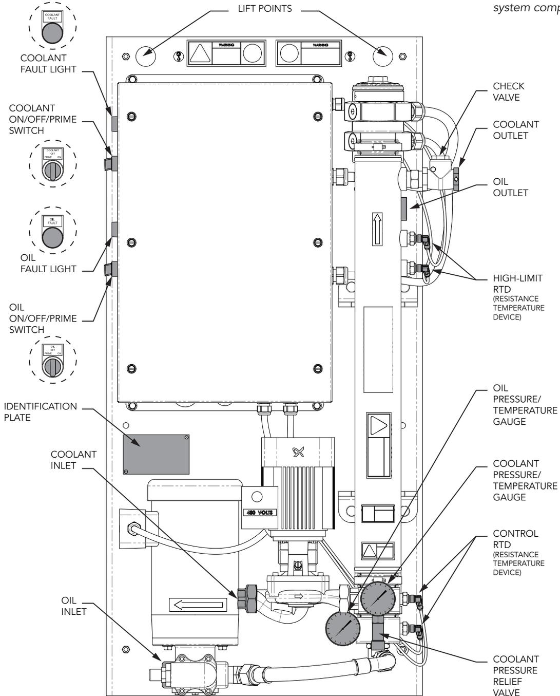
Figure 1. DLV heating system components.
