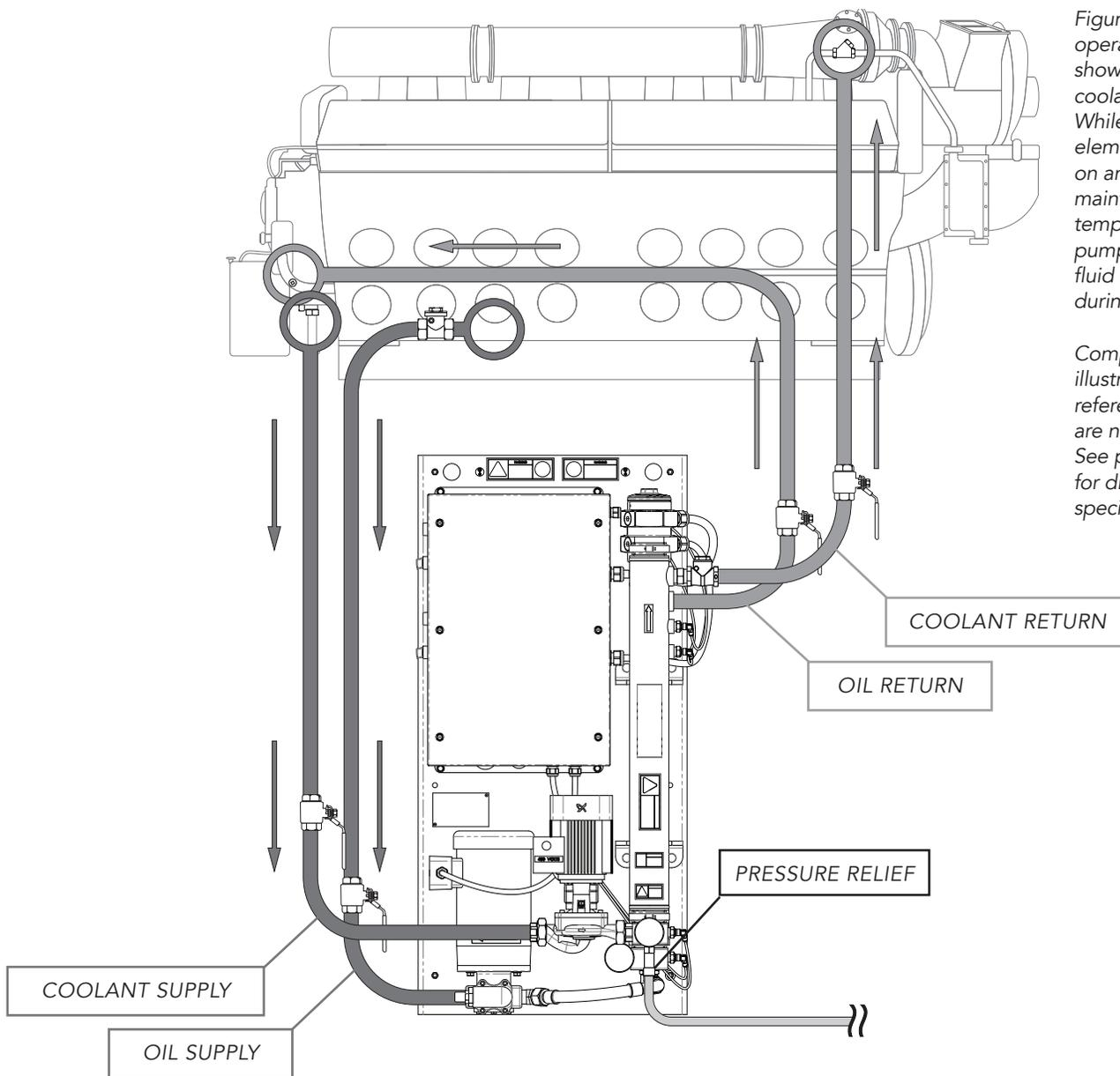
Figure 1. DLV operation overview, showing oil and coolant circulation. While the heating elements cycle on and off to maintain the preset temperature, the pumps circulate fluid continuously during operation.
