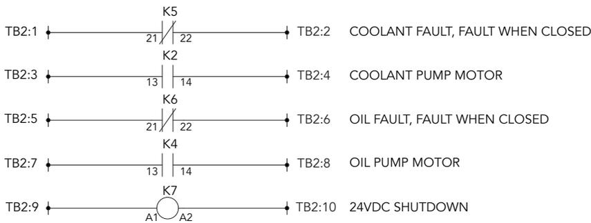
Figure 3. Customer interface connection wiring schematic for the DLV heating system.
