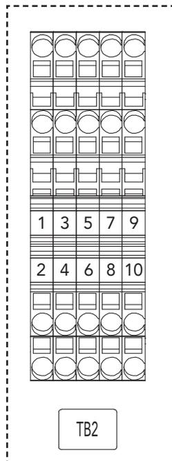
Figure 4. Customer interface connections (TB2) as shown in the DLV control box.
