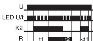
(green LED U/t illuminated). When the control contact K2 is closed, the set interval t1 begins (green LED U/t flashes slowly). After the interval t1 has expired, the output relay R switches into on-position (yellow LED
