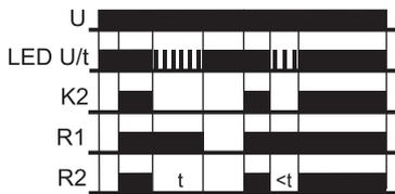
on-position (yellow LED R illuminated). If the control contact is opened, the instantaneous contact switches into off-position and the set interval t begins (green LED U/t flashes). After the interval t has expired (green LED U/t illuminated) the delayed contact switches into off-position (yellow LED R not illuminated). If the control contact is closed again before the interval t has expired, the interval already expired is erased and is restarted with the next cycle.
