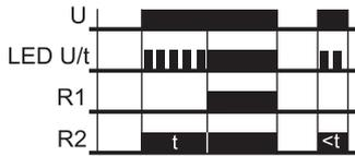
the set interval t begins (green LED U/t flashes). After the interval t has expired (green LED U/t illuminated) the delayed contact switches into on-position (yellow LED R illuminated).
