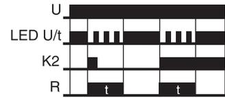
illuminated). When the control contact K2 is closed, the output relay R switches into on-position (yellow LED illuminated) and the set interval t begins (green LED U/t flashes). After the interval t has expired (green LED U/t illuminated) the output relay switches into off-position (yellow LED not illuminated). During the interval, the control contact K2 can be operated any number of times. A further cycle can only be started when the cycle run has been completed.
