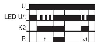
illuminated). When the control contact K2 is closed, the set interval t begins (green U/tLED flashes). After the interval t has expired (green LED U/t illuminated) the output relay R switches into on-position (yellow LED illuminated). This status remains until the control contact K2 is opened. If the control contact K2 is opened before the interval t has expired, the interval already expired is erased and is restarted with the next cycle.
