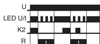
condition of the output relay R. When the control contact K2 is opened, the output relay switches into on-position (yellow LED illuminated) and the set interval t begins (green LED U/t flashes). After the interval t has expired (green LED U/t illuminated), the output relay switches into off-position
