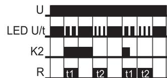
contact K2 is closed, the output relay R switches into on-position (yellow LED illuminated) and the set interval t1 begins (green LED U/t flashes slowly). After the interval t1
