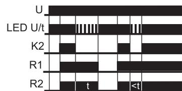
When the control contact K2 is closed, the output relays switch into on-position (yellow LED R illuminated). If the control contact is opened, the set interval t begins (green LED U/t flashes). After the interval t has expired (green LED U/t illuminated) the output relays switch into off-position (yellow LED R not illuminated). If the control contact is closed again before the interval t has expired, the interval already expired is erased and is restarted with the next cycle.
