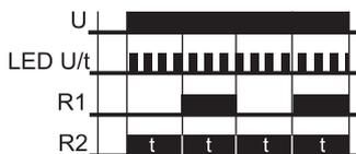
the set interval t begins (green LED U/t flashes). After the interval t has expired, the delayed contact switches into on-position (yellow LED R illuminated) and the set interval t begins again. After the interval t has expired, the delayed contact switches into off-position (yellow LED R not illuminated). The delayed contact is triggered at a ratio of 1:1 until the supply voltage is interrupted.
