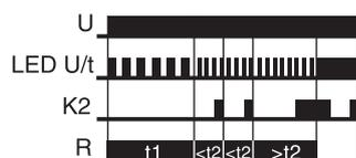
the interval  $t1$  has expired, the set interval  $t2$  begins (green LED  $U/t$  flashes fast). For the output relay to remain in on-position, the control contact  $K2$  must be closed and reopened within the set interval  $t2$ . If this does not occur, the output relay  $R$  switches into off-position (yellow LED not illuminated) and all further pulses at the control contact  $K2$  are ignored. To restart the function, the supply voltage must be interrupted and reapplied.
