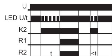
When the control contact K2 is closed, the set interval t begins (green LED U/t flashes). After the interval t has expired (green LED U/t illuminated) the output relays switch into on-position (yellow LED R illuminated). This status remains until the control contact is opened again. If the control contact is opened before the interval t has expired, the interval already expired is erased and is restarted with the next cycle.
