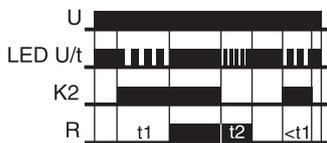
illuminated). When the control contact K2 is closed, the set interval t1 begins (green LED U/t flashes slowly). After the interval t1 has expired, the output relay R switches into on-position (yellow LED illuminated). When the control contact K2 is opened, the set interval t2 begins (green LED U/t flashes fast). After the interval t2 has expired, the output relay switches into off-position (yellow LED not illuminated).
