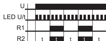
interval t has expired, the output relays switch into on-position (yellow LED R illuminated) and the set interval t begins again. After the interval t has expired, the output relays switch into off-position (yellow LED R not illuminated). The output relays are triggered at a ratio of 1:1 until the supply voltage is interrupted.
