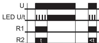
illuminated) and the set interval t begins (green LED U/t flashes). After the interval t has expired (green LED U/t illuminated) the output relays switch into off-position (yellow LED R not illuminated). This status remains until the supply voltage is interrupted. If the supply voltage is interrupted before the interval t has expired, the output relays switch into off-position. The interval already expired is erased and is restarted when the supply voltage is next applied.
