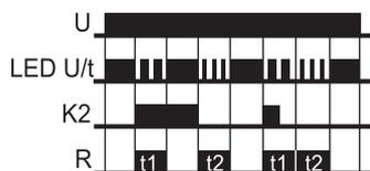
contact  $K2$  is closed, the output relay  $R$  switches into on-position (yellow LED illuminated) and the set interval  $t1$  begins (green LED  $U/t$  flashes slowly). After the interval  $t1$  has expired, the output relay  $R$  switches into off-position (yellow LED not illuminated).
