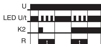
output relay R switches into on-position (yellow LED illuminated) and the set interval t begins (green LED U/t flashes). After the interval t has expired (green LED U/t illuminated) the output relay switches into off-position (yellow LED not illuminated).
