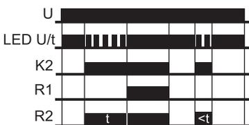
When the control contact K2 is closed, the instantaneous contact switches into on-position and the set interval t begins (green LED U/t flashes). After
