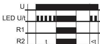
interval t has expired (green LED U/t illuminated) the output relays switch into on-position (yellow LED R
