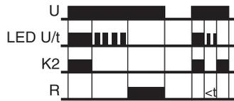
contact K2 is opened, the set interval t begins (green LED U/t flashes). After the interval t has expired the output relay switches into on-position (yellow LED illuminated). If the control contact K2 is closed before the interval t has expired, the interval already expired is erased and is restarted with the next cycle.
