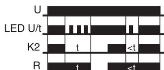
When the control contact K2 is closed, the output relay R switches into on-position (yellow LED illuminated). If the control contact K2 is opened, the set interval t begins (green LED U/t flashes). After the interval t has expired (green LED U/t illuminated) the output relay switches into off-position (yellow LED not illuminated).
