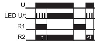
illuminated) and the set interval t begins (green LED U/t flashes). After the interval t has expired (green LED U/t illuminated) the delayed contact switches into off-position (yellow LED R not illuminated). This status remains until the supply voltage is interrupted.
