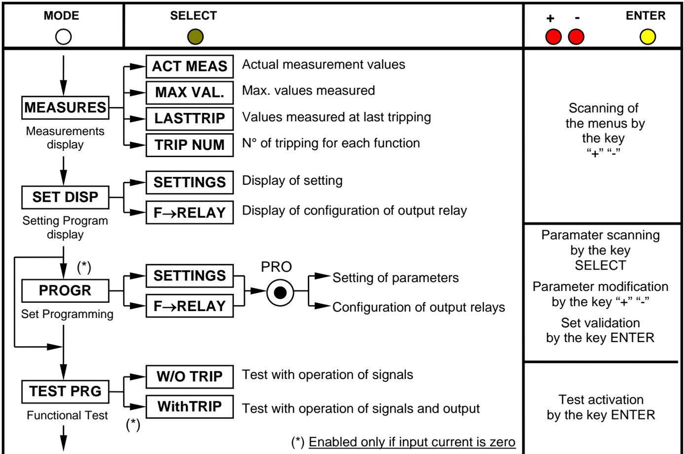
Pressing this button progressively selects between Measurements Display, Setting Display, Programming, and Test modes
