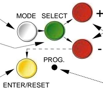
The + and - buttons are used to select the actual measurement or display desired when in Measurements Display or Settings Display modes. When in Program mode, these buttons increase or decrease the value of the displayed setting.
